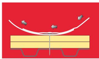
With Firestone's symmetrical Wide-Weld<sup>™</sup> Seam Technology, a 5" weld area completely surrounds the fastener, distributing uplift forces uniformly along all edges of the fastening system and eliminating peel forces of conventional single-weld
