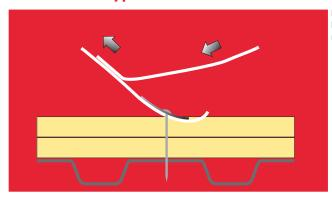
In a conventional asymmetrical TPO seam, less than half of the seam is welded. As a result, wind uplift ratings are limited.
